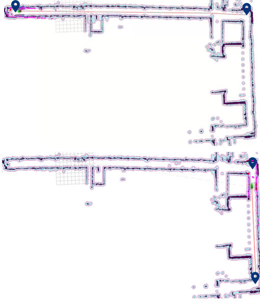
Figure 2: RViz navigation visualization of the route segments, showing the occupancy grid map, robot localization, and executed path between reference points.
